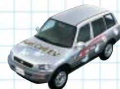
In an exhibition parade in Osaka, Japan, Toyota demonstrates its in-house-developed FCHV, equipped with an original fuel cell stack and hydrogen-absorbing alloy tank.
